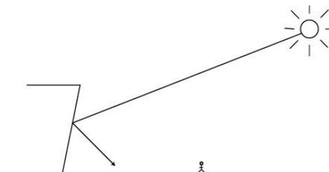
A façade or canopy that slopes back from the vertical can reflect high angle sun along the ground. This is of particular concern as motorists will not be expecting it, the high angle sun is brighter, and the sun is less likely to be intercepted by other buildings before it reaches the glass.
