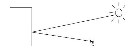
A façade that slopes forward, so that the top of the building forms an effective overhang, is unlikely to cause significant reflected solar glare.
